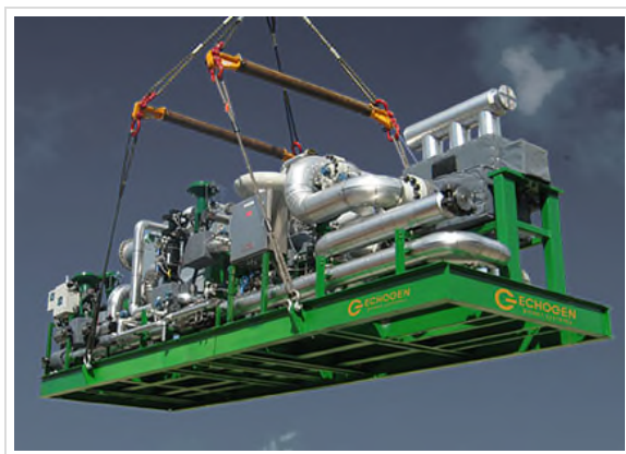
Figure 4. Echogen EPS 100 Process skid (left) and Power Skid Right (Courtesy Echogen Power Systems and Dresser-Rand)
