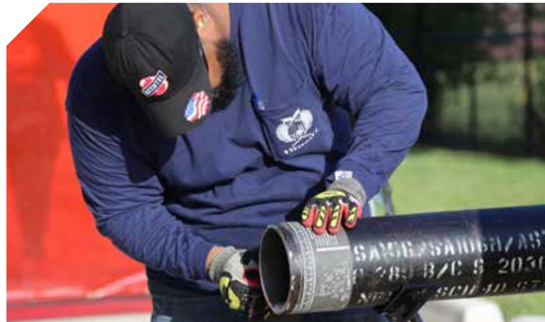
Student applies his training instruction by using a wraparound to make a pipe bandsaw cut.
