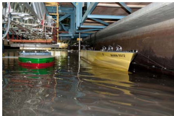
Figure 5: MARIN tests with moored vessel and passing ship under drift angle
