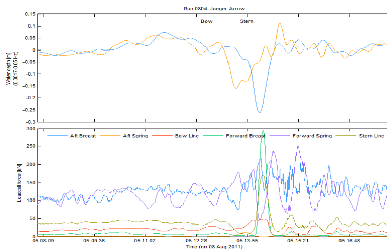
Figure 3: Water draw down and mooring line loads measured at the Nieuwe Maas river location
