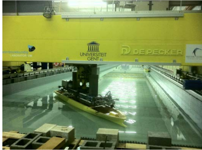
Figure 2: Fully automated systematic model tests at FHR in Borgerhout
