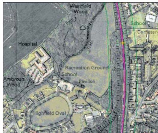
Figure 3. Example of 1:10,000 Raster Mapping Transparently Overlaid over 25 cm Resolution
